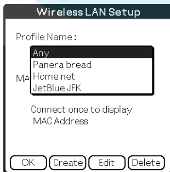
Figure 15-17: On CLIÉs with a CompactFlash Wi-Fi card, you must select the proper profile when using a protected network.
